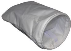
FiltaSolid filter elements remove particulates from your fuel. The 800, 900 and 999 series offer 80.0%, 90.0% and 99.9% efficiency on particles between 1 and 800µm (microns).
