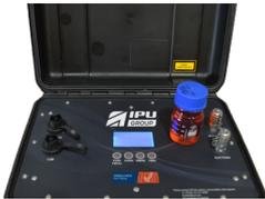
The DieselCheck portable diesel analyser quickly, accurately and economically checks a sample's water and particulate content and fuel density.
